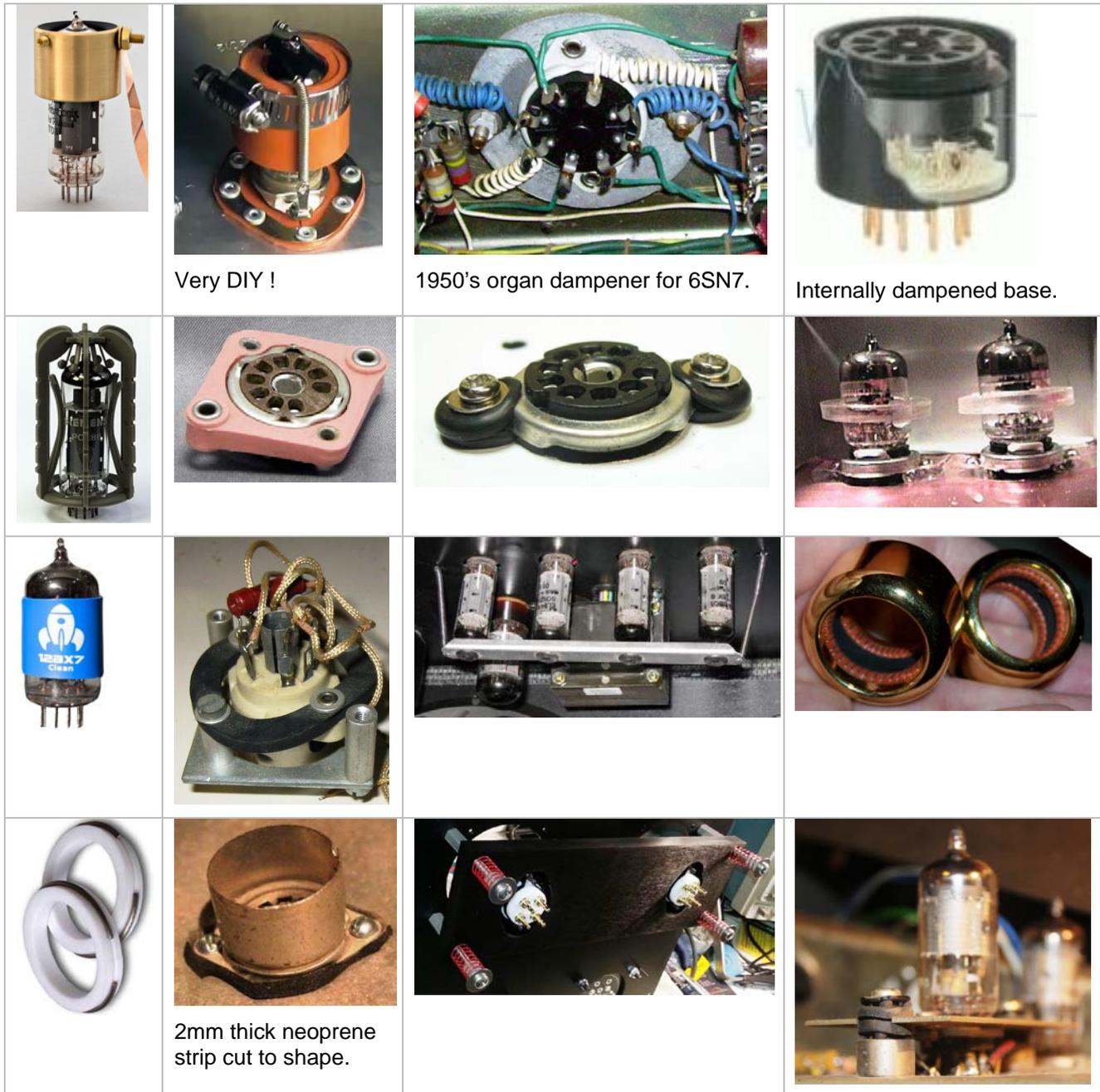
A variety of valve-based vibration attenuators.
