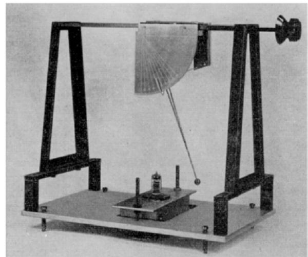
Fig. 6—Apparatus for measuring microphony by shock excitation
